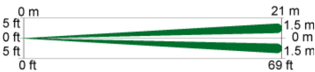
Top View Optional Long Range Coverage: 21 m x 3 m (70 ft x 10 ft)
